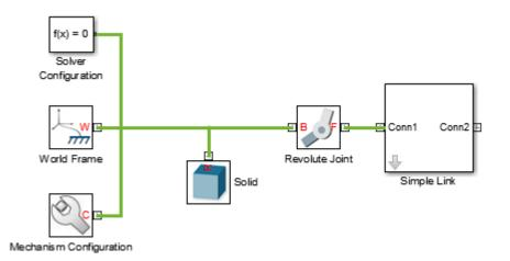
**6** In the Solid block dialog box, specify the following parameters. This block connects rigidly to the World frame and therefore has no effect on model dynamics. You can leave the inertia parameters in their default values.
