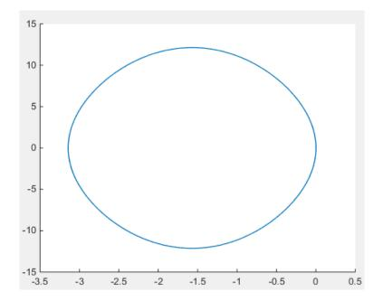
Try simulating the model using different starting angles. You can change the starting angle in the **State Targets** > **Position** menu of the Revolute Joint block dialog box. The figure shows a compound phase plot for starting angles of -80, -40, 0, 40, and 80 degrees.
