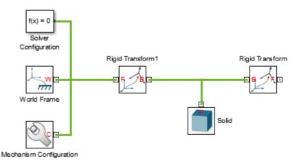
5 In the Solid block dialog box, specify the following parameters. Later, you define the MATLAB variables shown using a Subsystem block that contains the Solid and Rigid Transform blocks. Among its advantages, this approach enables you to update variables used in multiple blocks from a single place—the Subsystem block dialog box.
